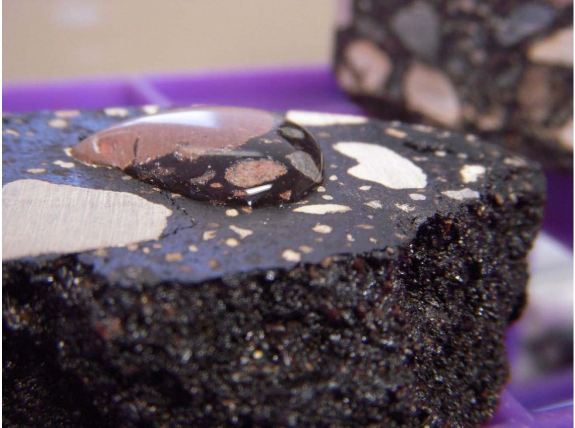
Figure 9. Water on an Asphalt Concrete Core.
