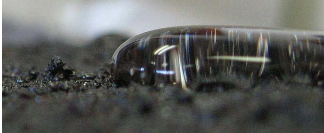
Figure 8. Water Drop On Dry Asphalt Concrete Core.
